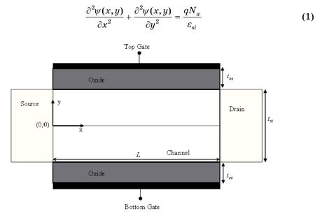
Fig. 1 – Schematic structure of DG MOSFET
