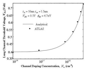
Fig. 3 - Long channel threshold voltage with channel doping
