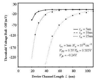
**Fig.** 5 –  $\Delta V_{th}$  with channel length for  $t_{ox} = 1$  nm
