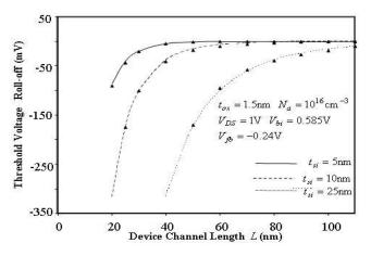
**Fig.** 6 –  $\Delta V_{th}$  with channel length for  $t_{ox} = 1.5$  nm
