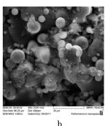
Fig. 1 – SEM-images of plasma sprayed hydroxyapatite coating without TMP (a) and after TMP anneal by 800  $^{\circ}{\rm C}$  (b)
