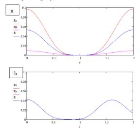
**Fig. 9** – Reflection of calculated two-layer nanoporous coating on glass ( $n_s = 1.52$ ) on different angles of light incidence: 45° (a) and 0° (b). Matched parameters:  $a_1 = 1.318$ ,  $a_2 = 1.178$ ,  $n_1 = 1.086$ ,  $n_2 = 1.339$
