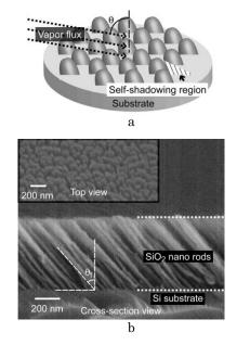
**Fig.** 8 – Schematic of oblique-angle deposition (a). Top and cross-sectional views of a SEM for a  $SiO_2$  nanorod layer (b) [3]
