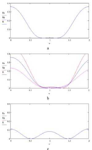
**Fig.** 7 – Calculated two-layer coating reflection for two substrates: with  $n_s=4$  (angles of light incidence equals 0° (a) and 45° (b)) and  $n_s=2$  at normal incidence of light (c)
