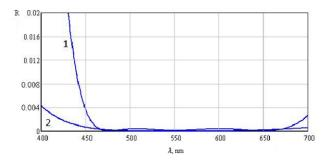
**Fig. 10** – The spectral dependencies of the reflectance R for coated glass substrate ( $n_s = 1.52$ ) at normal light incidence. Curve 1 – four-solid-layer antireflective coating with optical thicknesses  $\lambda/4 - \lambda/2 - \lambda/4 - \lambda/4$  with corresponding refractive indexes  $n_1 = 1.38$ ,  $n_2 = 2.35$ ,  $n_3 = 1.548$ ,  $n_4 = 1.38$ . Curve 2 – two layer coating,  $n_1 = 1.1$ ,  $n_2 = 1.356$ .
