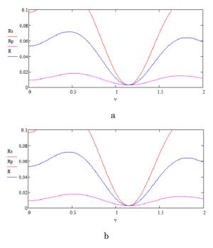
Fig. 6 – Calculated optical reflection for two-layer antireflection coating. Angles of light incidence equals 0° (a) and 45° (b).  $n_1=1.38$ ,  $n_2=1.701$ ,  $n_s=1.52$
