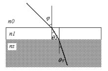
Fig.  $3-\mbox{The scheme of a single-layer antireflection coating.}$
