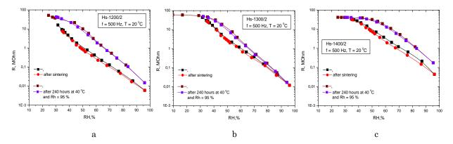
Fig. 2 – Exploitation properties of MgO-Al<sub>2</sub>O<sub>3</sub> ceramics sintered at 1200 °C (a), 1300°C (b) and 1400°C (c)
