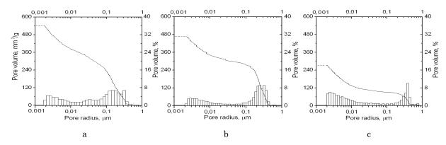
Fig. 1 – Pore size distributions of MgO-Al<sub>2</sub>O<sub>3</sub> ceramics sintered at 1200 °C (a), 1300 °C (b) and 1400 °C (c)
