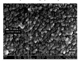
Fig. 3 – In this scanning electron microscopy micrograph can be seen the minimum structural element (30 nm) of the deposited material
