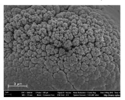
Fig. 2 – Scanning electron microscopy image of the structure deposited out of solution composition: 0.02 M chloride copper(II), 0.5 M ammonia, 0.075 M ethylene glycol, 0.3 M potassium bromate, laser power 1300 mW, the scanning rate 0.01 mm/s, the substrate Polycore VK-96
