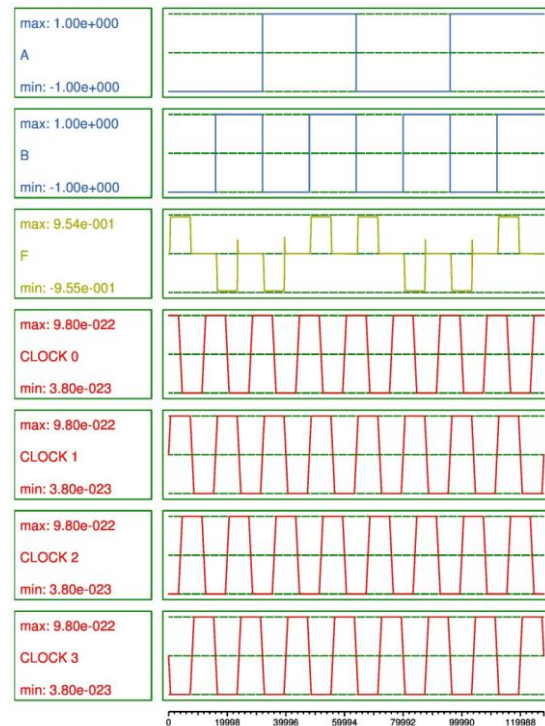
Fig. 5 – Simulation results of QCA Akers two input XOR gate
