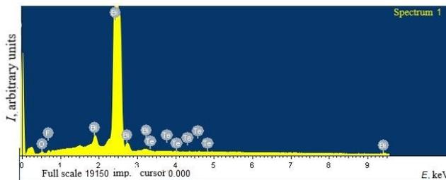
**Fig. 3** – The electronic spectrum of Bi (0.150 at. % Te)
