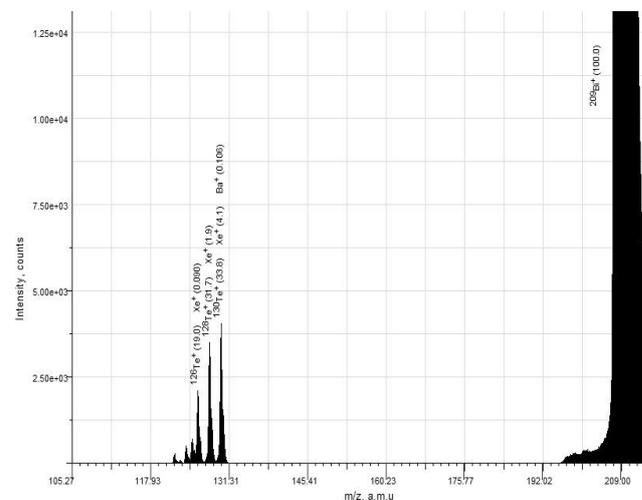
Fig. 2 – Mass spectrum of Bi (0.150 at. % Te). Combined cathode. The material of cathode wall is Al. Pressure 1.6 Torr. Gas mixture composition: Ar – 69.70 %, He – 30 %, H<sub>2</sub> – 0.30 %
