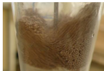
Fig. 2 – Fluidized bed with partial swirling
