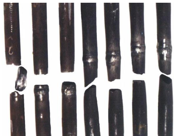
Fig. 4 - Section-type specimens (welded coiled tubing) after the tensile test
