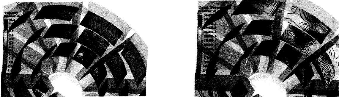
a) b) Fig. 2 Distribution of absolute velocity and pressure in the between blades channels of the pump impeller
