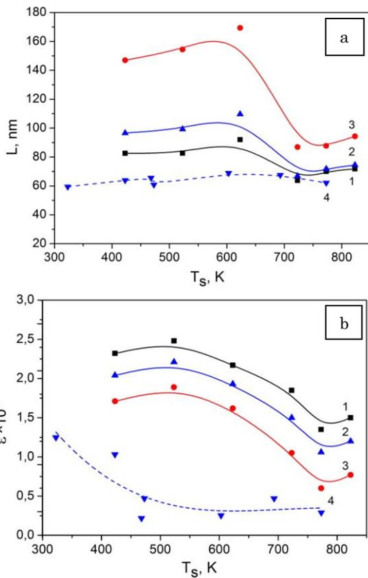
**Fig. 2** – The effect of the substrate temperature  $T_s$  on the CSD size (a) and the microdeformation grade (b) of the films  $Zn_{1-x}Mn_xTe$  (1-3) and ZnTe (4). The approximation is done according to Cauchy (1), Gauss (3), and to the method of three-fold convolution (2)
