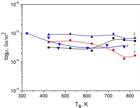
**Fig. 3** – Dependence of the dislocation concentration on the substrate temperature in  $Zn_{1-x}Mn_xTe$  (1-3) and  $ZnTe$  (4) films: at the subgrain boundaries (1), in their bulk (2) and the general dependence (3, 4) using the reflexes (111)-(222).
