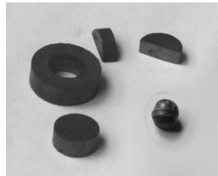
Fig. 2 – Samples of EDS consolidated \text{Si}_3\text{N}_4 –TiN, TiN – \text{TiB}_2 compositions
