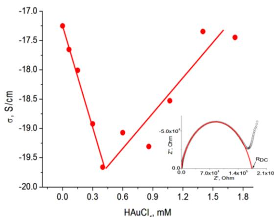
**Fig. 3** – DC conductivity of CS / AuNP's films as a function of the of the  $\text{HAuCl}_4$  concentration obtained from impedance measurements at room temperature. Insert shows complex impedance spectra
