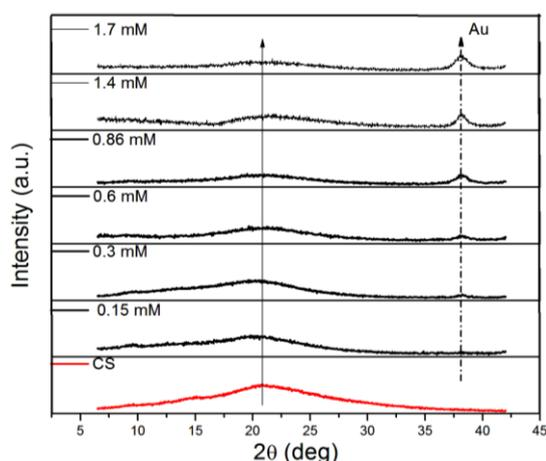
**Fig. 1** – XRD pattern of films obtained from solution with different  $\text{HAuCl}_4$  concentration
