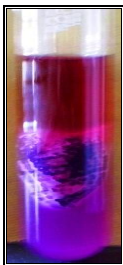
Fig. 2 – Cobalt tartrate crystals under variation of upper reactant conc. is 0.5 M
