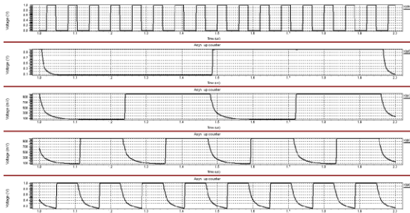
Fig. 9 – Simulation output of 4 bit hybrid asynchronous up counter
