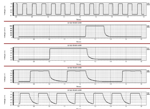
Fig. 14 – Simulation output of a 4 bit hybrid synchronous-asynchronous decade counter
