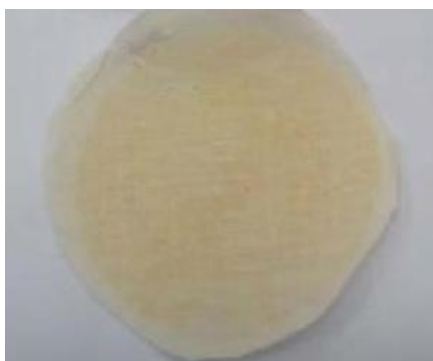
Fig. 5 – Sample S1 with yellow color imparted by nanosilver
