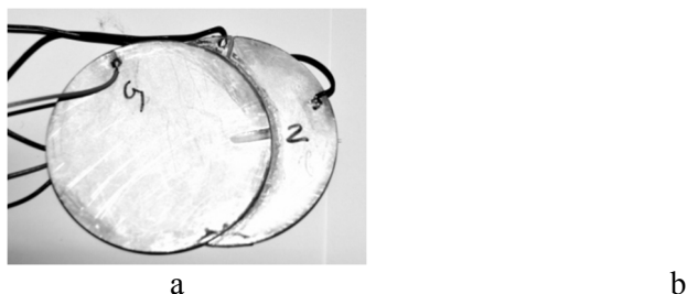
Fig. 1 – Symmetric bimorph element with a shift piezo elements (a) and the amplitude-frequency characteristics (b)
