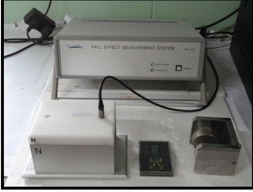
Fig. 1 – Hall Effect instrument experimental set-up
