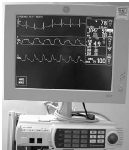
Figure 1.8 – Integrated monitoring system displaying ECG and heart rate (beats/min), non-invasive blood pressure (mmHg), capnograph and end tidal carbon dioxide (kPa), pulse oximeter waveform and saturation (%)
