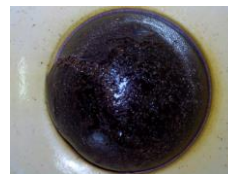
Fig. 1 – The dried gel of NiFe 2 O 4 sample
