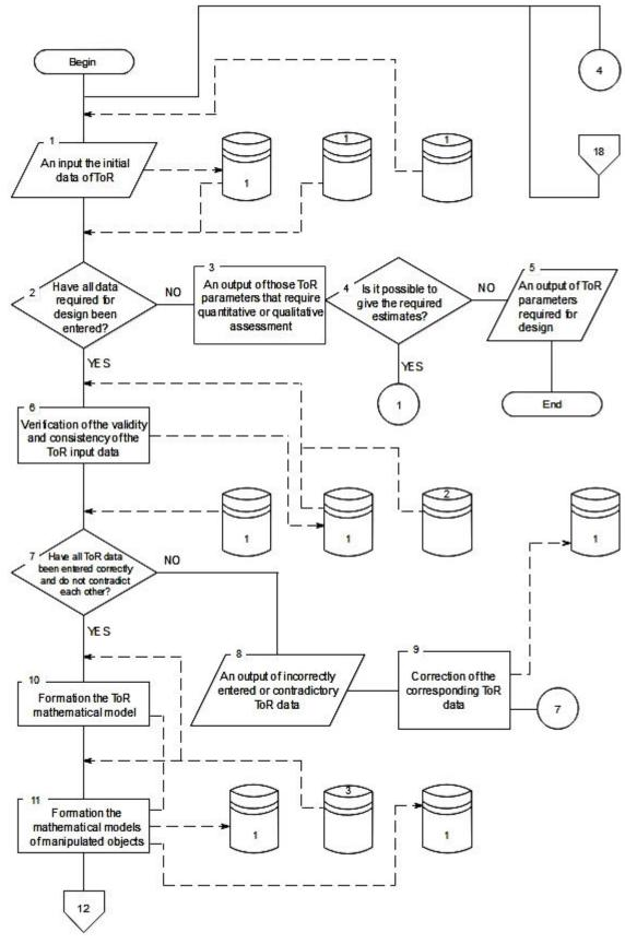
Figure1 - Fragment of the automated design flowchart
