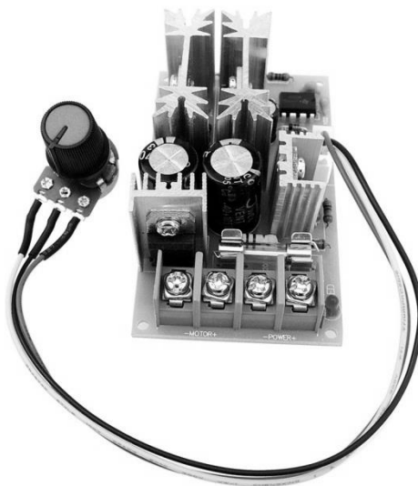
Figure 1. PWM Controller- part of the automated complex for research tensoresistive properties of nanostructured film
