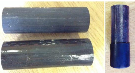
Figure 2. Preparation of the corroding samples: original iron bar, bar coated with PCB lacquer, coated bar with set heat shrink tubing
