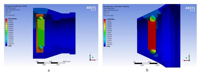
Figure 6 – Deformations of the bearing supports 45-216 (a) and 45-276214 (b) as a result of axial preloading, radial force and rotation of the rotor
