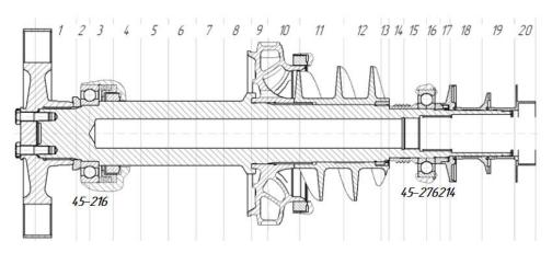
Figure 1 - Design scheme of the oxidizer turbopump rotor
