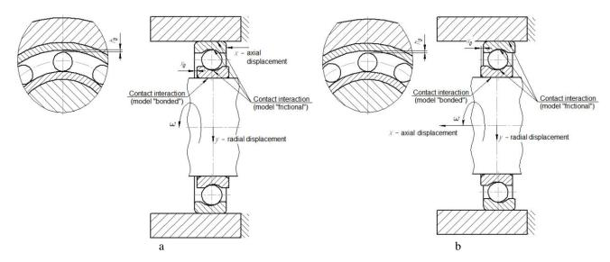
Figure 2 – Design scheme of the bearing supports 45-216 (a) and 45-276214 (b)
