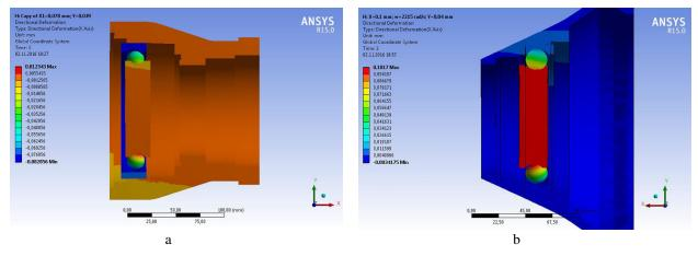
Figure 7 – Isosurfaces of axial displacements for the bearing supports 45-216 (a) and 45-276214 (b)
