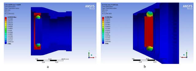
Figure 4 - Deformations of the bearing supports 45-216 (a) and 45-276214 (b) as a result of axial preloading
