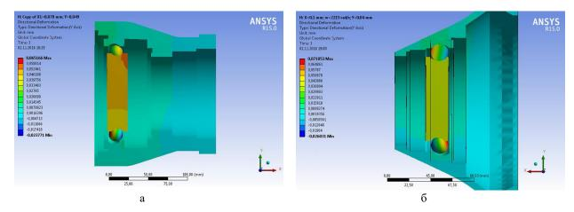
Figure 8 – Isosurfaces of radial displacements for the bearing supports 45-216 (a) and 45-276214 (b)
