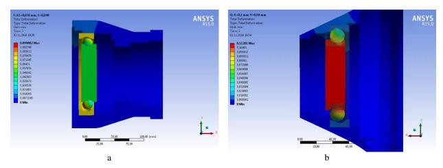
Figure 5 – Deformations of the bearing supports 45-216 (a) and 45-276214 (b) as a result of axial preloading and radial force
