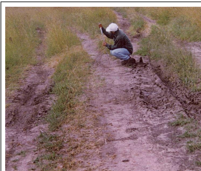
Photos 5 and 6 show the measurement of soil compaction. Medani Bhandari is measuring soil compaction inside the off-road tract (off road damaged area, where still off road is continue).
