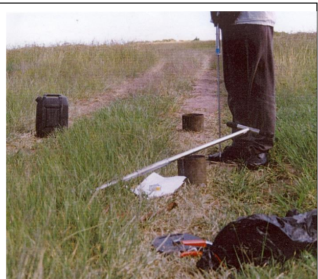
Photos 5 and 6 show the measurement of soil compaction. Medani Bhandari is measuring soil compaction inside the off-road tract (off road damaged area, where still off road is continue).
