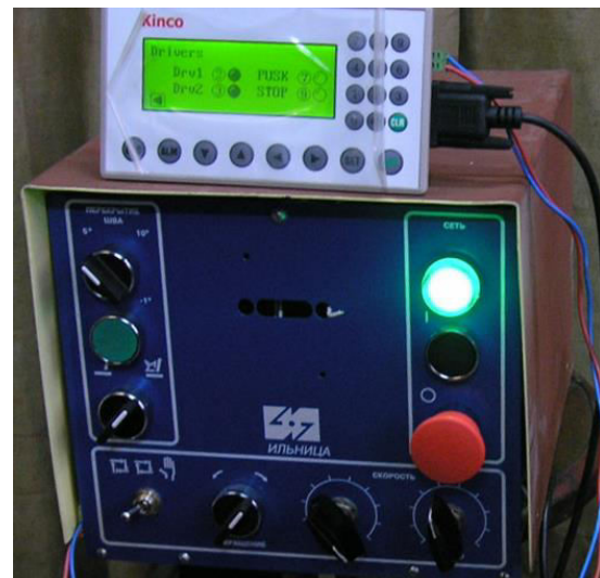
Figure 2 – The appearance of the control panel stepper motor
