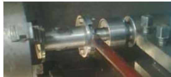
Figure 7 – Calibration of the instrument for torque measurement
