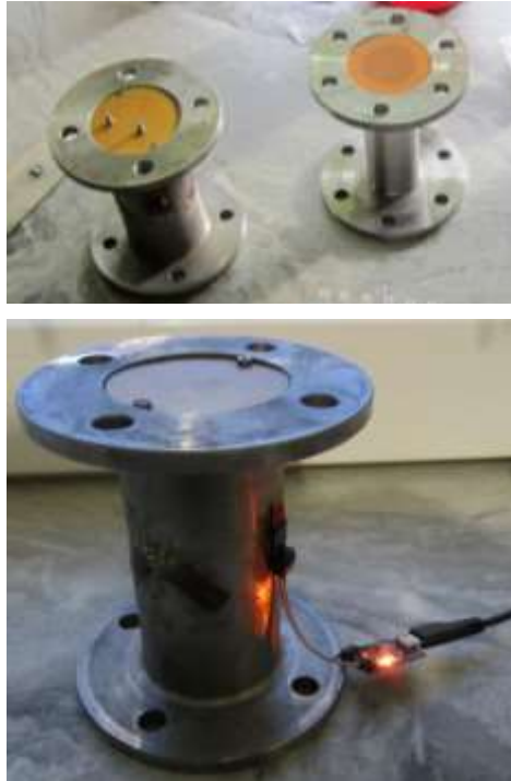
Figure 6 – Strain-gauge clutch for torque measurement
