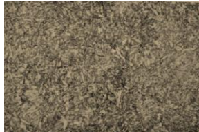
Figure 4 – Microstructure of steel HNM5 after standard heat treatment, x500
