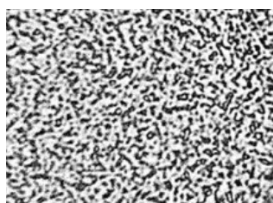
Figure 7 – Microstructure of steel AISI 420 after quenching at 1000 °C (×500)
