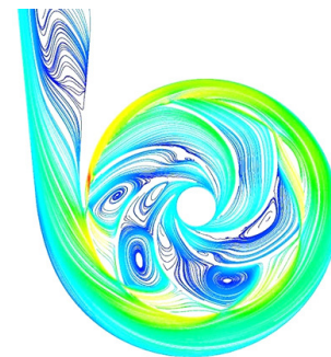
Fig. 6. The structure of the fluid flow in the flowing part of the pump at flow rate 0.6 Q_{opt}
