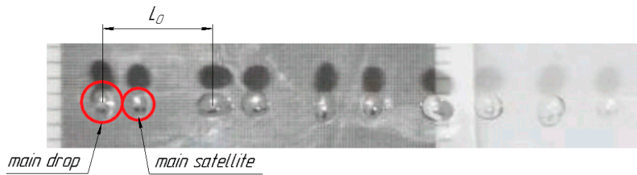
Figure 2. The decay of the jet into drops at the frequency of 240 Hz.
