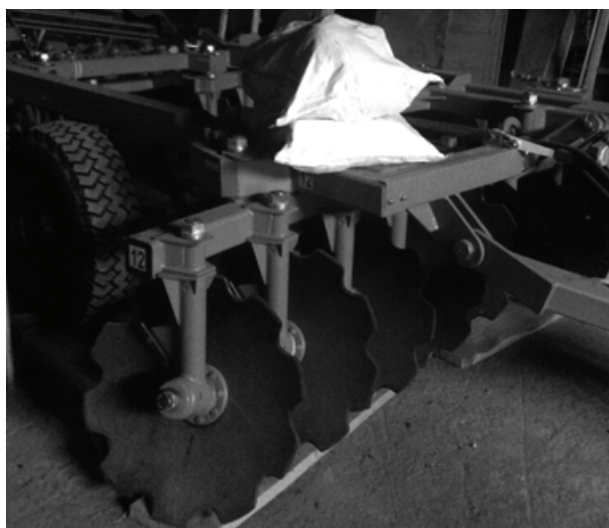
Fig. 3. Adjusting the disking depth with the additional load on the UDA-3.1 implement. According to the methodology all the data were examined separately
