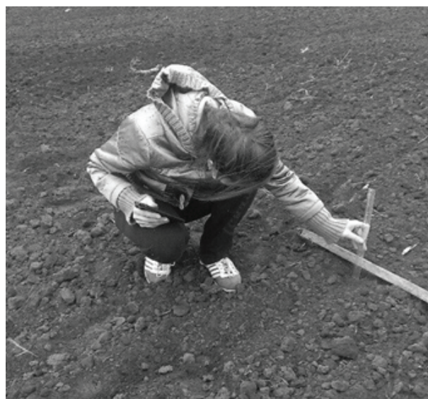
Fig. 5. Determination of the ridges height on the soil surface after disking
