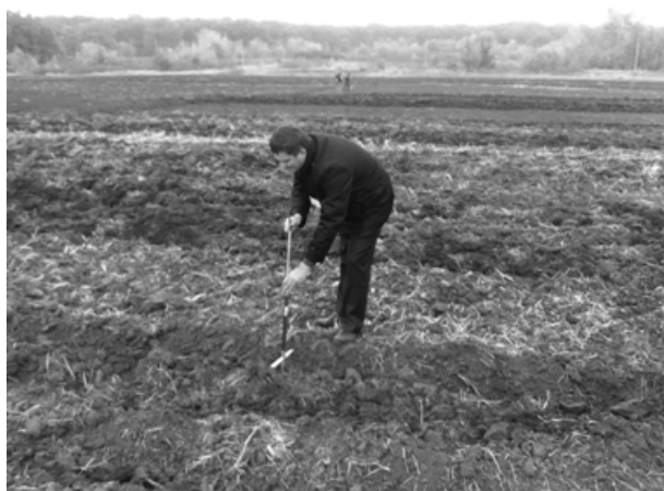
Fig. 4. Determination of the depth evenness after disking
