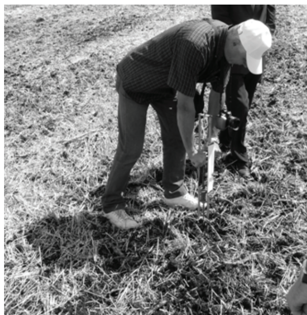
Fig. 6. Defining the penetration resistance of the soil
