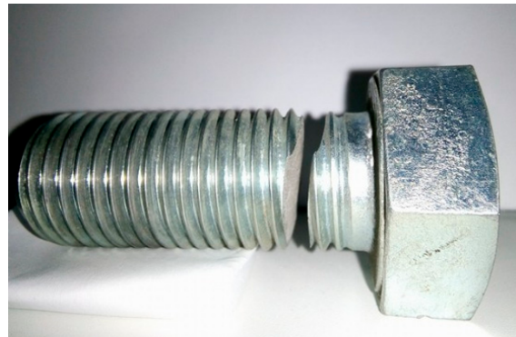
Figure 1. Operational fracture of high-strength screw.
