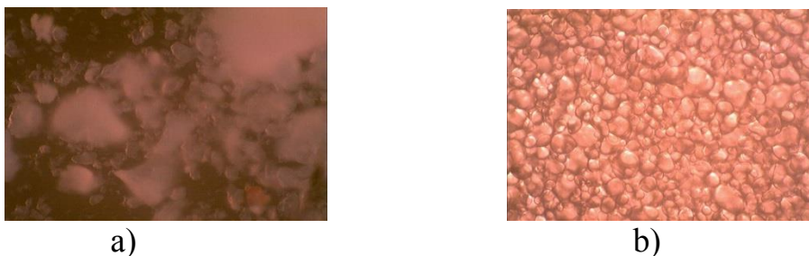
Figure. 1 – Micrographs of the original starch (a) and starch nitrate witch obtained by nitration in 98% nitric acid (b).
