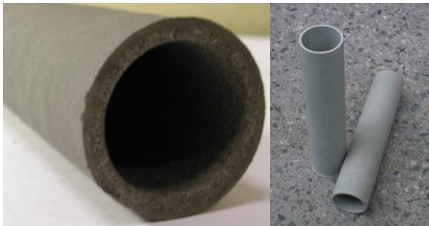
Figure 8 – Multilayer PPM made of the steel powder BBS15 \varnothing 40 \times 220 mm using the radial isostatic pressing method
