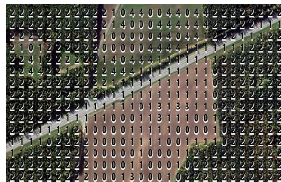
Fig. 6. The Identification result of the image frames of the region at the initial values of the RGB-component images weights
