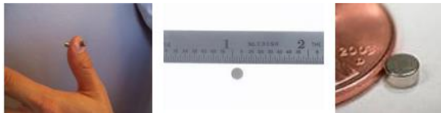
Figure 7. Magnets fallen out of large toy components
