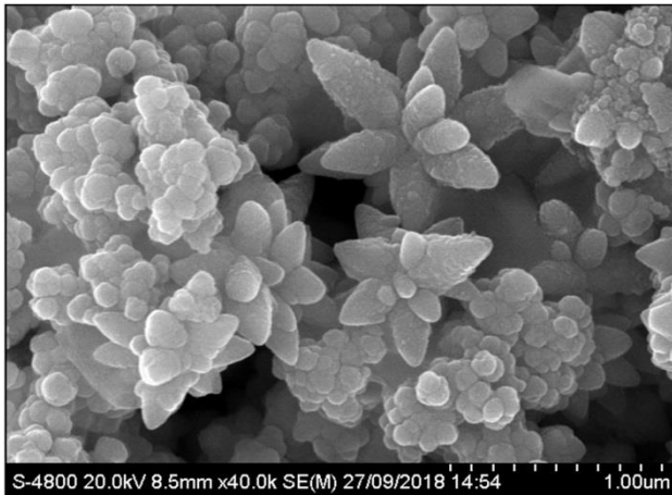
Fig. 3 – FESEM micrograph of Cd_{1-x}Mn_xS thin films deposited at x = 0.2
