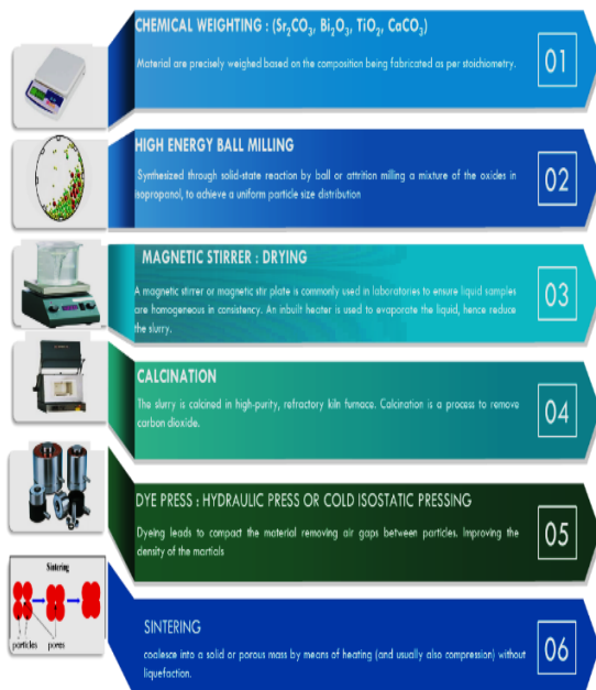
Fig. 2 – Flow chart: preparation of lead-free piezoelectric ceramics
