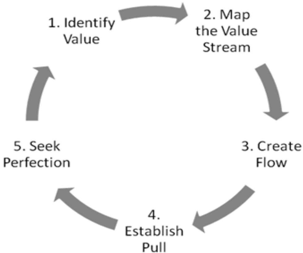
Fig 3.1.3 An illustration of the lean management five steps thought process. (Womack and Jones, 1996)
