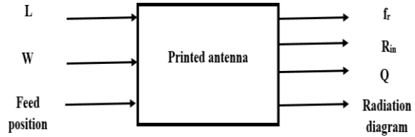
Fig. 1 – Operating characteristics of the printed antenna
