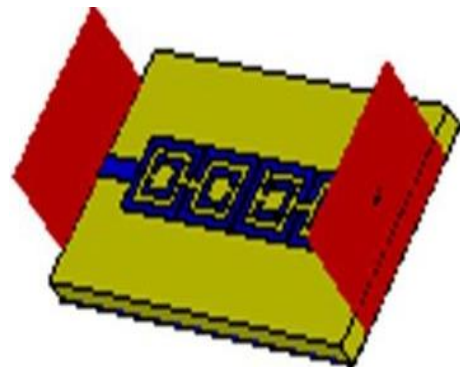
Fig. 4 – The 3D geometry of the band-pass filter
