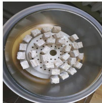
Figure 4 – The process of determining the degree of moisture absorption of a product made of shavings and dry adhesive mixtures
