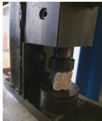
Figure 3 – Determining the compressive strength of wood chips and dry mixes
