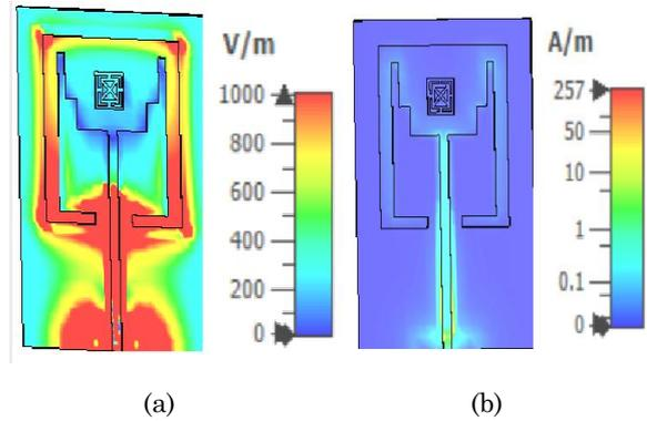
Fig. 6 – (a) Electric field distribution (b) Magnetic field distribution
