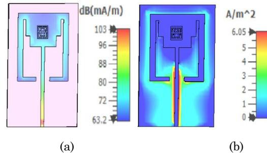
Fig. 7 – (a) surface current distribution (b) Current density distribution
