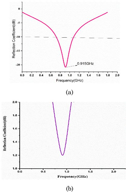
Fig. 3 – a) s11 parameter results of proposed antenna, (b) VSWR
