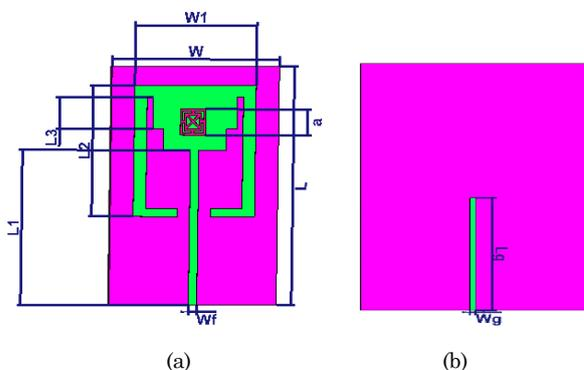
**Fig. 1** – Dimensional parameters of proposed antenna, (a) front view, (b) rear view
