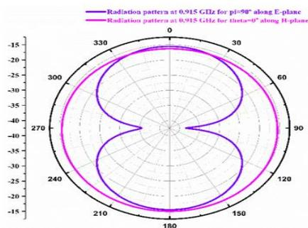
Fig. 5 – Radiation pattern along E- and H-planes at 0.915 GHz
