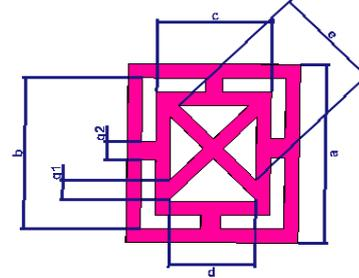
**Fig. 2** – Specifications of squared split ring resonator
