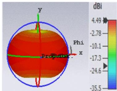
Fig. 4 – Gain obtained at 0.915 GHz frequency
