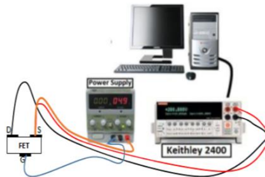
Fig. 2 – Circuit for measuring the I-V characteristic of OFET in ammonia vapor presence
