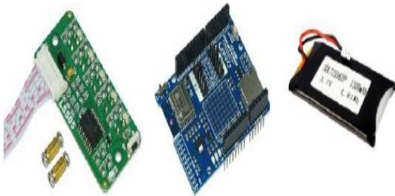
Fig. 6 – Line Sensor, Wi-Fi Module & LiPo Battery
