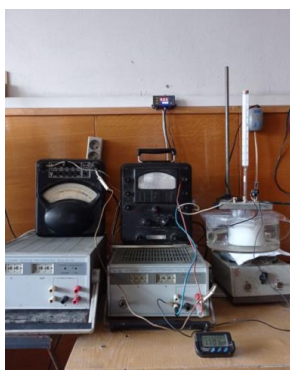
Fig. 1 – Installation for electrochemical synthesis of nanopowders
