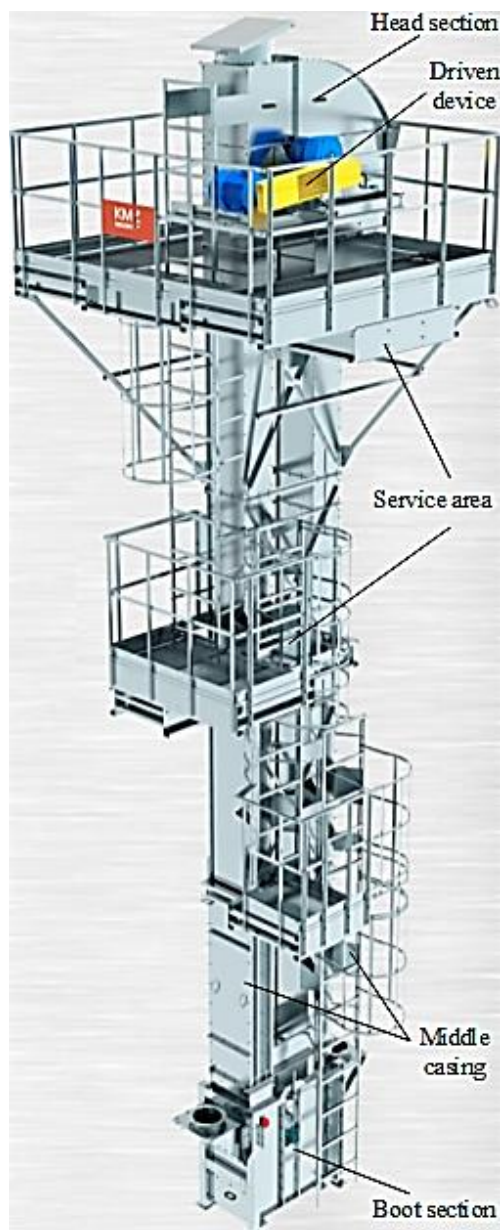
Figure 1 – Components of a bucket elevator
