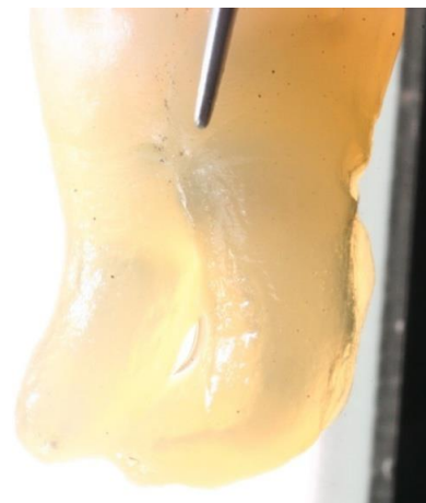
Figure 6 – Partial dye retention “Indian Ink” in the simulated resorption zone
