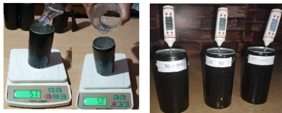
Fig. 1 – Experiment Set-up for mixed of paraffin wax and glycerine in different portions
