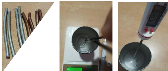
Fig. 2 – Experimental set-up of paraffin wax and glycerine blend with Aluminium and Copper fins
