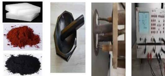
Fig. 3 – Experimental set-up of the blending of Paraffin wax with Iron (III) Oxide and Copper Oxide in different percentages ( x = 0, 0.05, 0.1, 0.5 ) and study of its characteristics.
